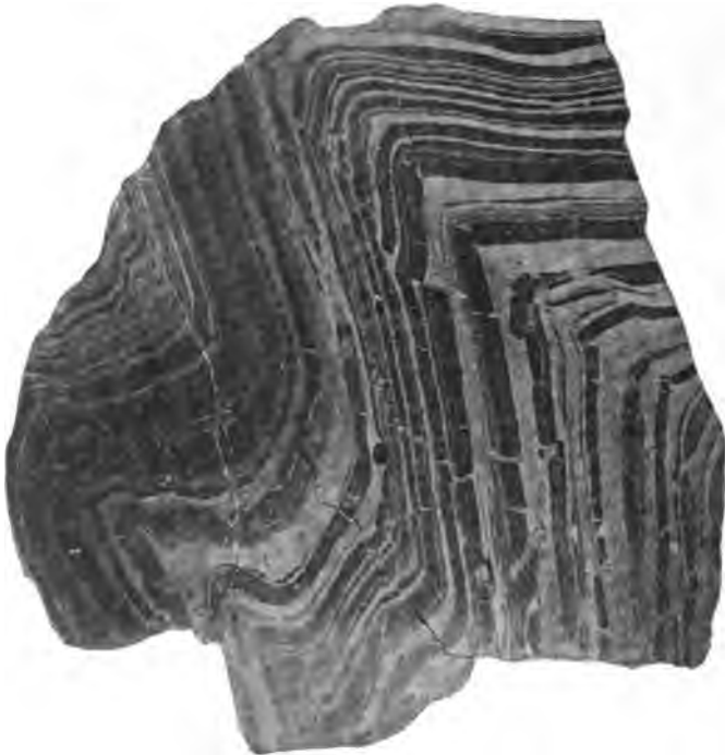
FIG. 187. — Folded and fractured iron ore and jaspilite, Lake Superior region. About \frac{1}{4} natural size
