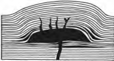
FIG. 216. — Diagrammatic vertical section of a laccolith (Gilbert). The full black indicates igneous rock
