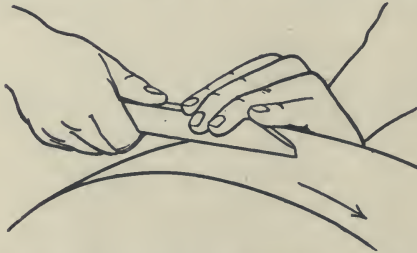
FIG. 56. — GRINDING TOP OF ROUND-NOSE TOOL ON GRINDSTONE
