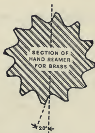
FIG. 19.—TEETH OF HAND REAMER WITH NEGATIVE RAKE.
