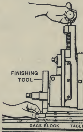
FIG. 25. — GAGE BLOCK TO SET PLANER TOOL.
