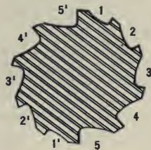
FIG. 51. — DIAGRAM OF REAMER SHOWING PRINCIPLE OF IRREGULAR SPACING.
