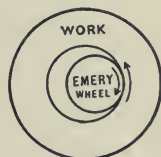
FIG. 21. — DIRECTION OF ROTATION OF WORK AND WHEEL FOR INTERNAL GRINDING.
