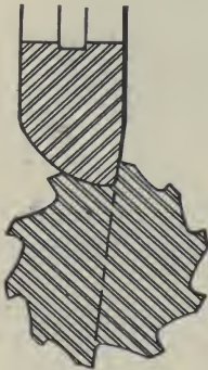
FIG. 48. — FORM OF FLUTE IN REAMER FOR GENERAL WORK. TEETH RADIAL. IRREGULARLY SPACED.
