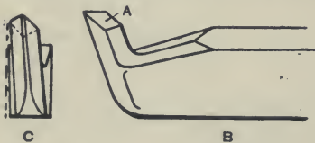
FIG. 15. — LEFT DIAMOND-POINT TOOL FOR STEEL OR WROUGHT IRON.
