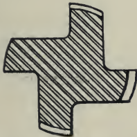
FIG. 43. — TAP GROOVED WITH SPECIAL DOUBLE-ANGLE TAP CUTTER, RADIAL TEETH.
