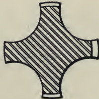
FIG. 44. — COMMERCIAL TAP GROOVED WITH CONVEX CUTTER.
